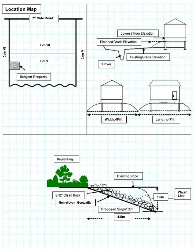
\*Slopes must be 3:1 or gentler unless there is not enough space, the rise is less than 1m, or it is replacing a vertical wall.
