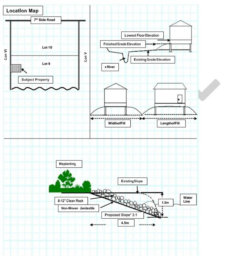
\*Slopes must be 3:1 or gentler unless there is not enough space, the rise is less than 1m, or it is replacing a vertical wall.
